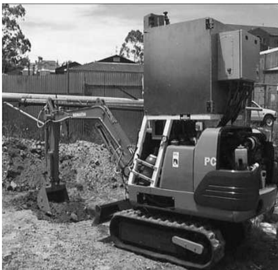
Figure 2: The robotic excavator in a trench-forming task[19].
