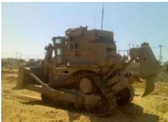
Figure 4: Robotic bulldozer for Military application[21]
